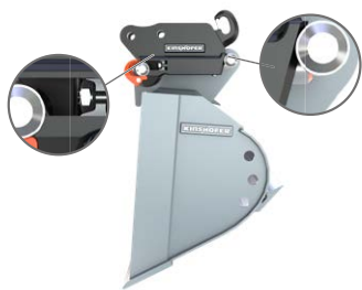
Safely locked. Indicator pin is driven in.
